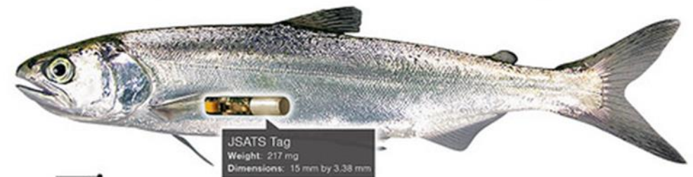
Injectable Acoustic Fish Tracking Tag
